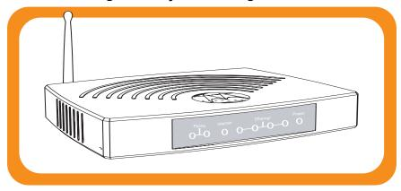
Power – When the power light stops blinking and is a solid green, this indicates that your Vonage Device has started up properly. Note that both the power light and the phone light must be solid in order to make a phone call.
